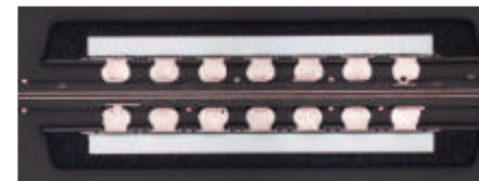
Double sided assembly - CSP
